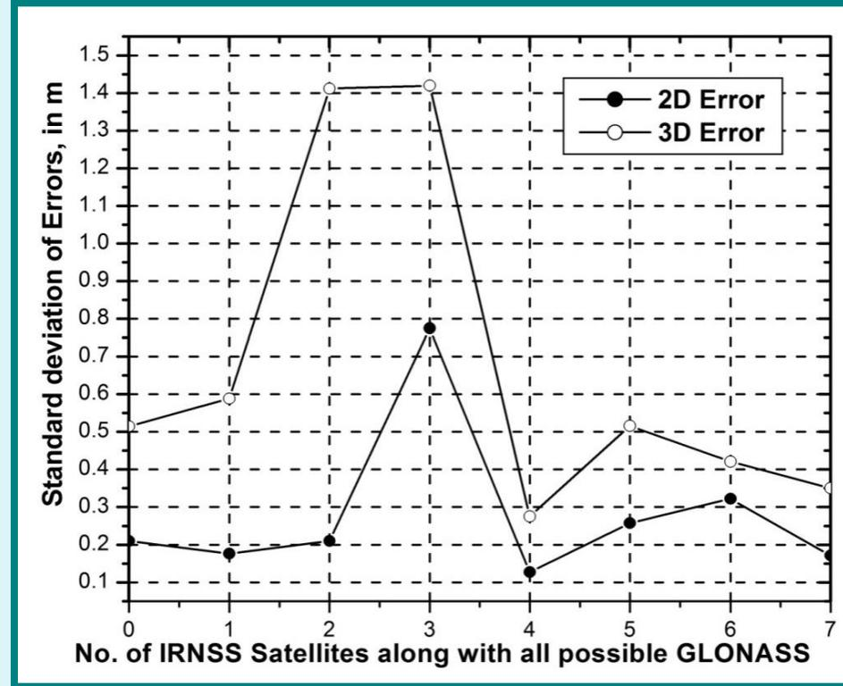
Variation of average errors and standard deviation of error with increasing number of IRNSS/ NavIC satellites with all available 09 GLONASS satellites (Date: 28/03/2019; Location: Burdwan)
