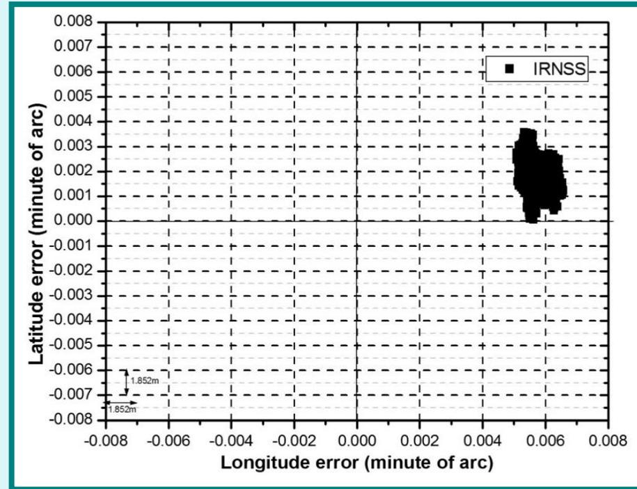
**IRNSS position solution errors (open sky); 27 January, 2019; one-hour data at 1 Hz rate, Burdwan, India. Dark lines indicate the reference coordinates**
