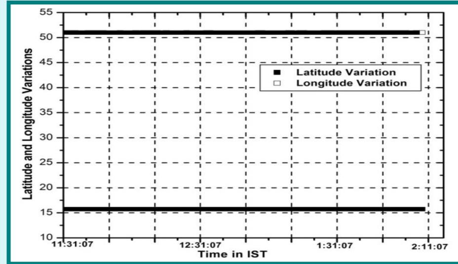
Solution Coordinates in constraint condition (urban canyon) in GLONASS+NavIC operation
