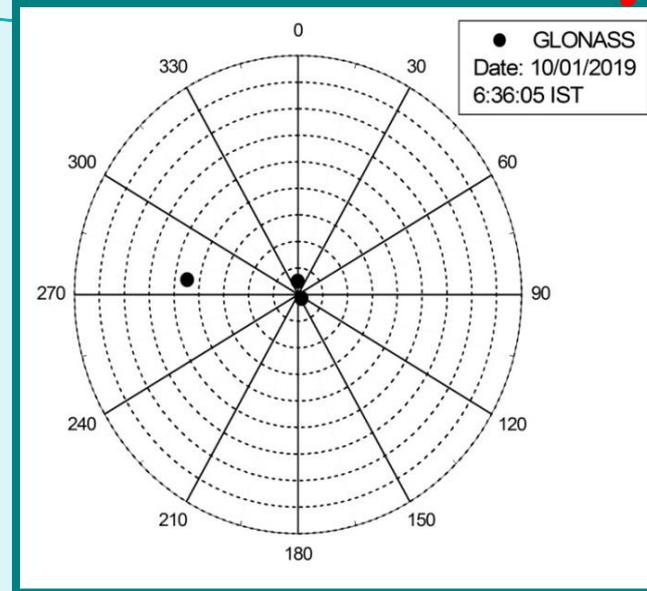
GLONASS skyplot when GLONASS alone could not provide position solution (10/01/2019; 6:36:05 IST)
