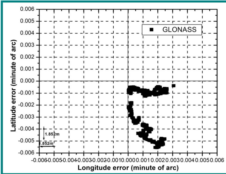
**GLONASS position solution errors (open sky); 10 January, 2019; one-hour data at 1 Hz rate, Burdwan, India. Dark lines indicate the reference coordinates**
