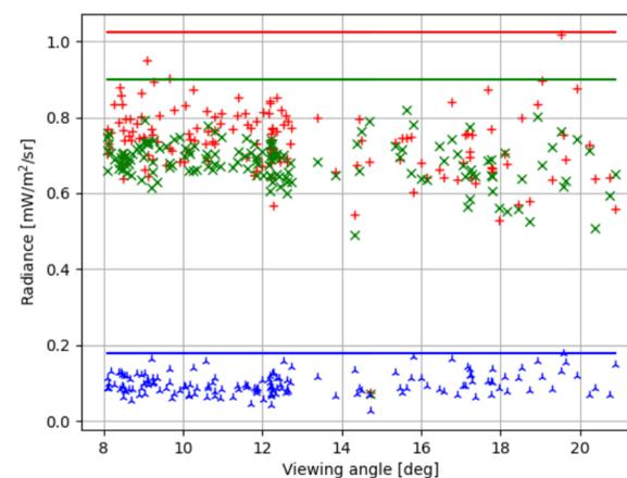
Figure 5: Angular emission of a single light source in the city of Timmins. The lines correspond to the value 3 standard deviation above the average for each band.
