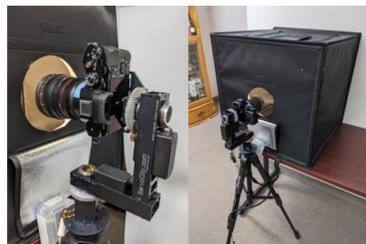
Figure 3: The camera is attached to a motorized mount that allows taking multiple images of the reference surface at different viewing angles, thereby simulating a larger, more uniformly lit surface.
