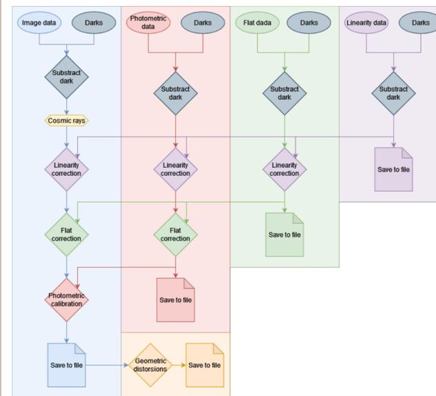
Figure 5: Complete calibration pipeline.
