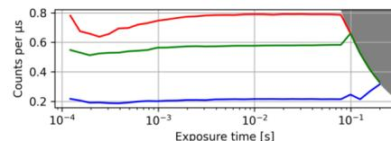
Figure 2: Digital number average rate for various exposure times. The three curves are for the three colour channels of the camera: red, green and blue, from top to bottom. The different levels are caused by the colour of the light source used for the test. The grey zone is the saturation area. One can notice the decrease in sensitivity for short exposure times.
