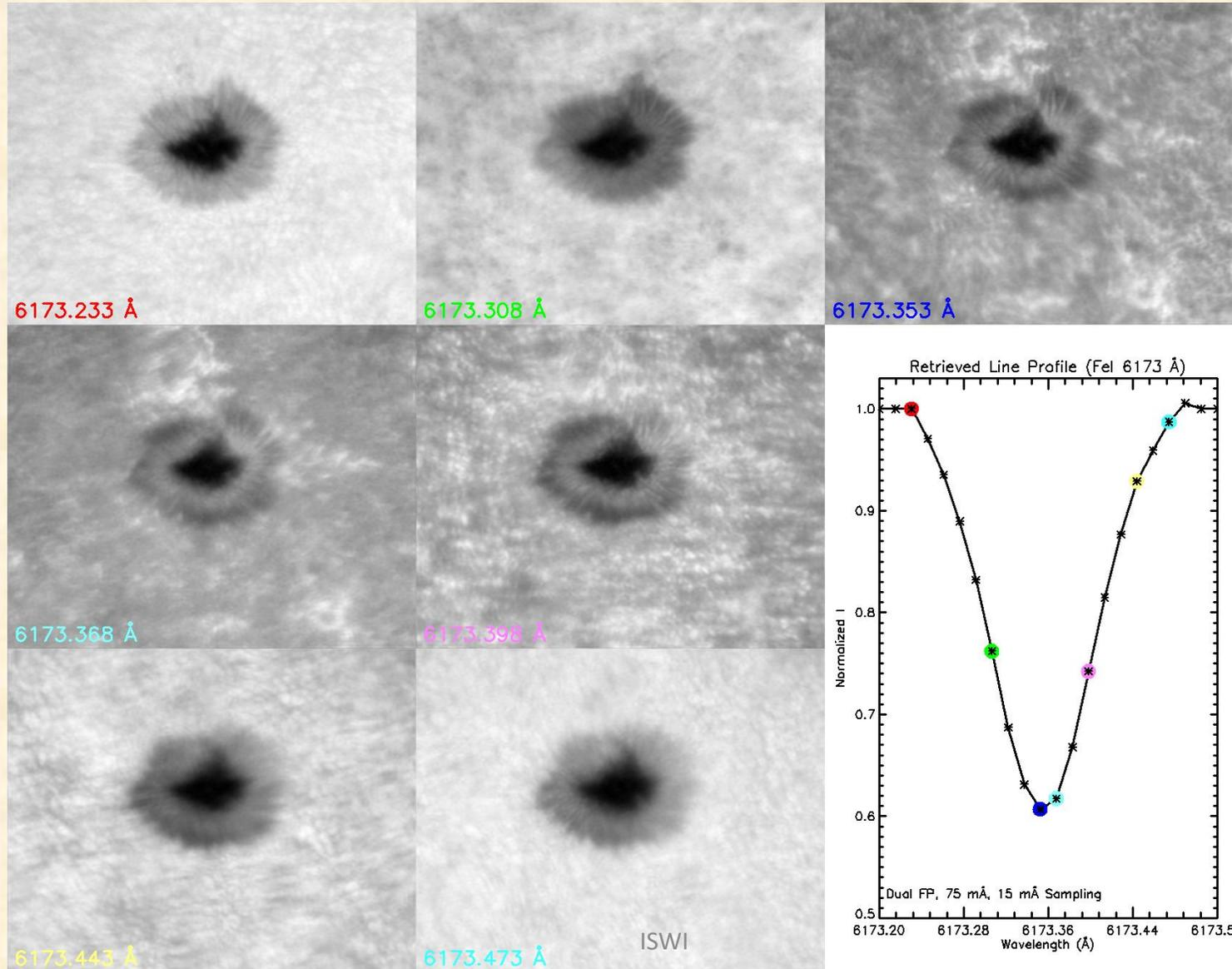
Fabry-Perot Narrow band imager; typical tuning result: 22 Wavelength positions along the 617.3 nm line profile with 15 mÅ steps
