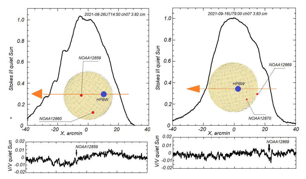
Stokes I and V records of transits of the Sun on 2021-08-26 and 2021-09-16 over RT-32 antenna beam. LNSP4, channel 7, 3.82 cm. Some side lobes of the antenna diagram and small polarization of rather weak ARs are clearly seen.
