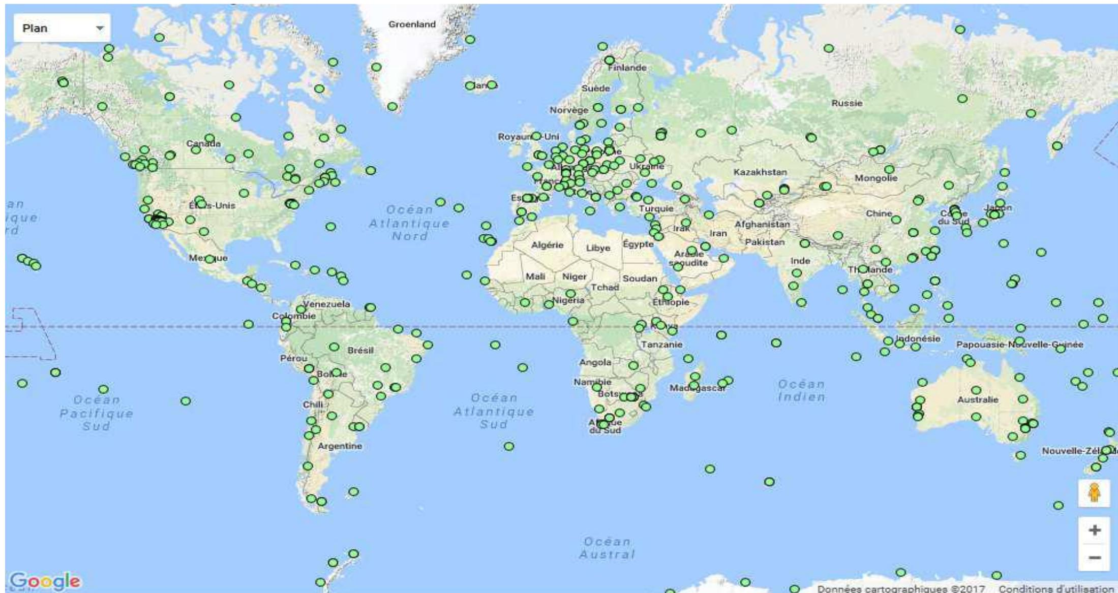
**IGS network is a global network of 513 permanent and continuously operating stations of geodetic quality**
