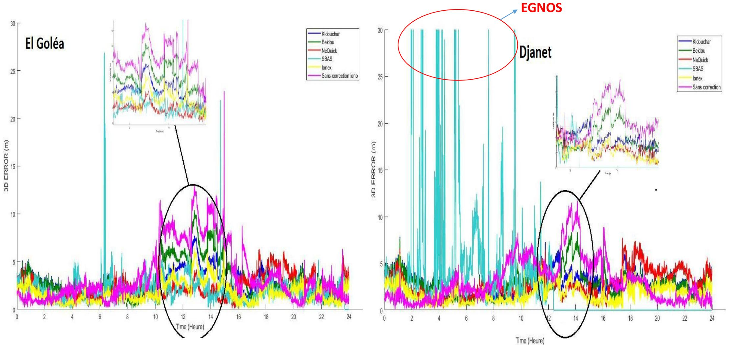
3D error (with zoom) in position errors from 12:00 to 14:00
