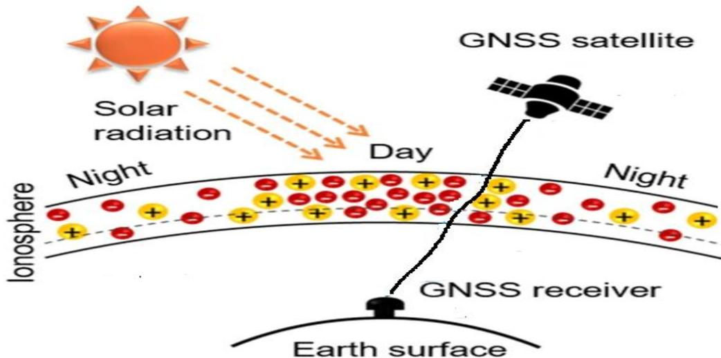
→ Ionospheric delay contributes to the general GPS error budget in the range of 40–60 m during daytime and 6–12 m at night.
