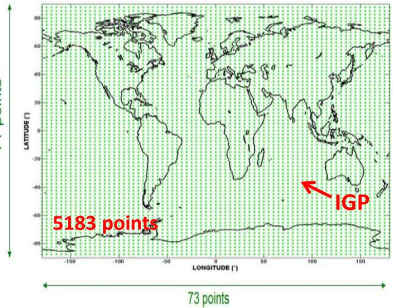
(IONEX: Ionospheric Grid Points 2,5°x5°)
