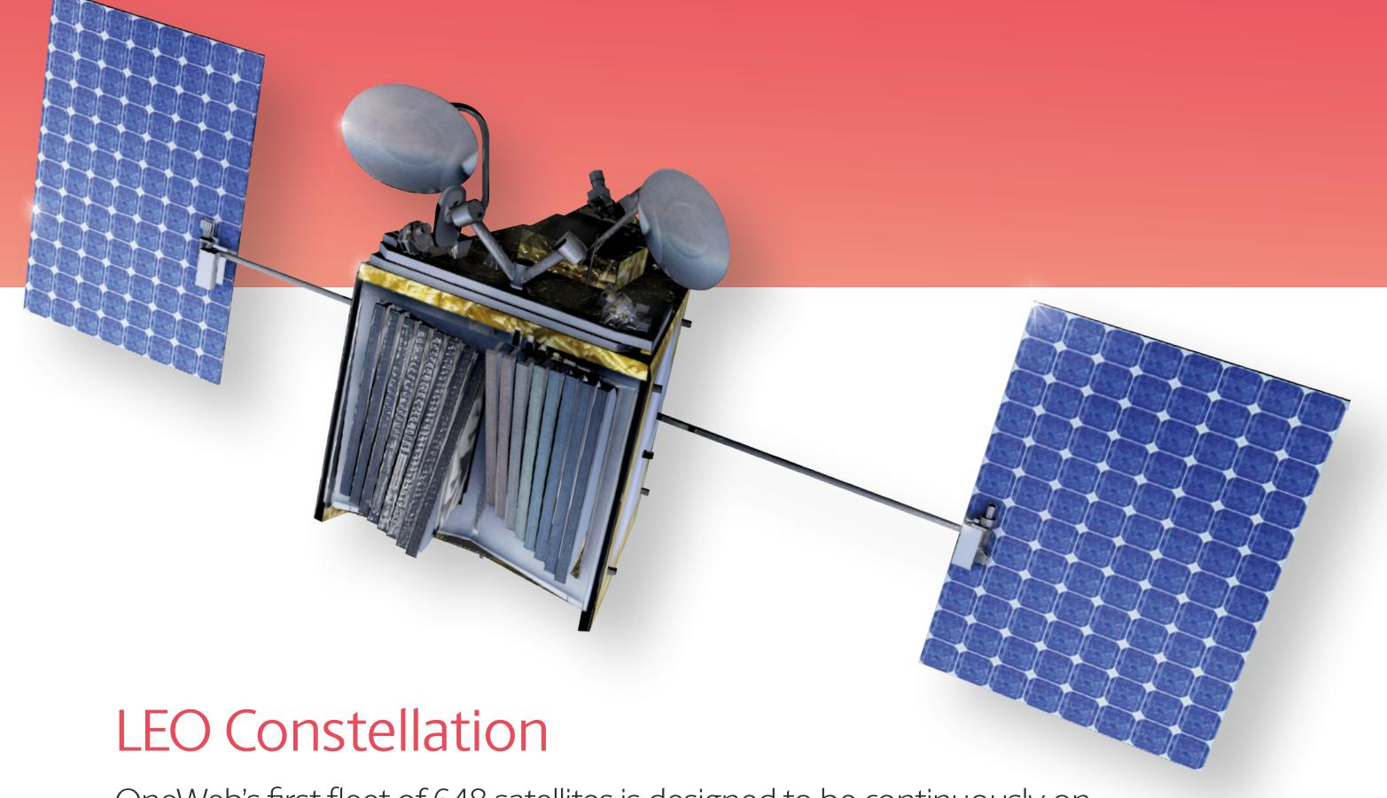
OneWeb's first fleet of 648 satellites is designed to be continuously on the move, travelling around the Earth every 90 minutes along 12 orbital planes at 1,200km from Earth which is 30x closer than GEO networks.
