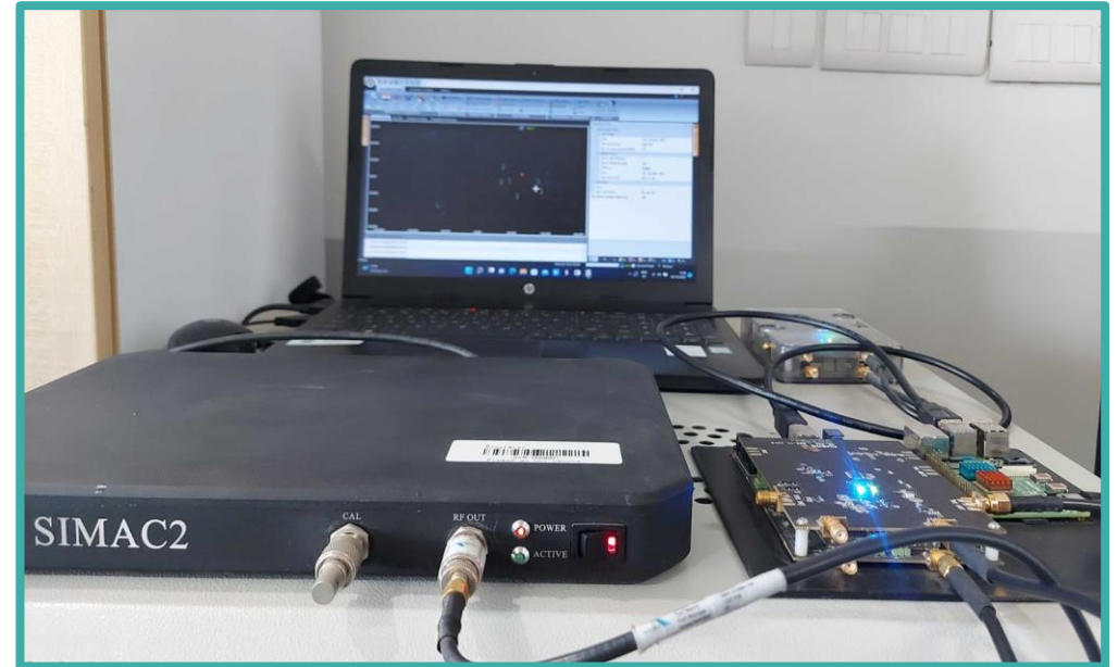
Fig 5. NavIC-R Receiver hardware setup
