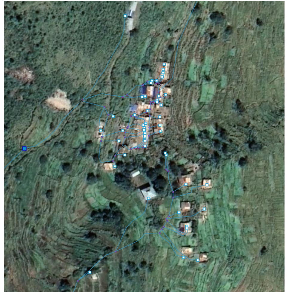
Water supply project designed using survey data from Low-Cost GNSS System
