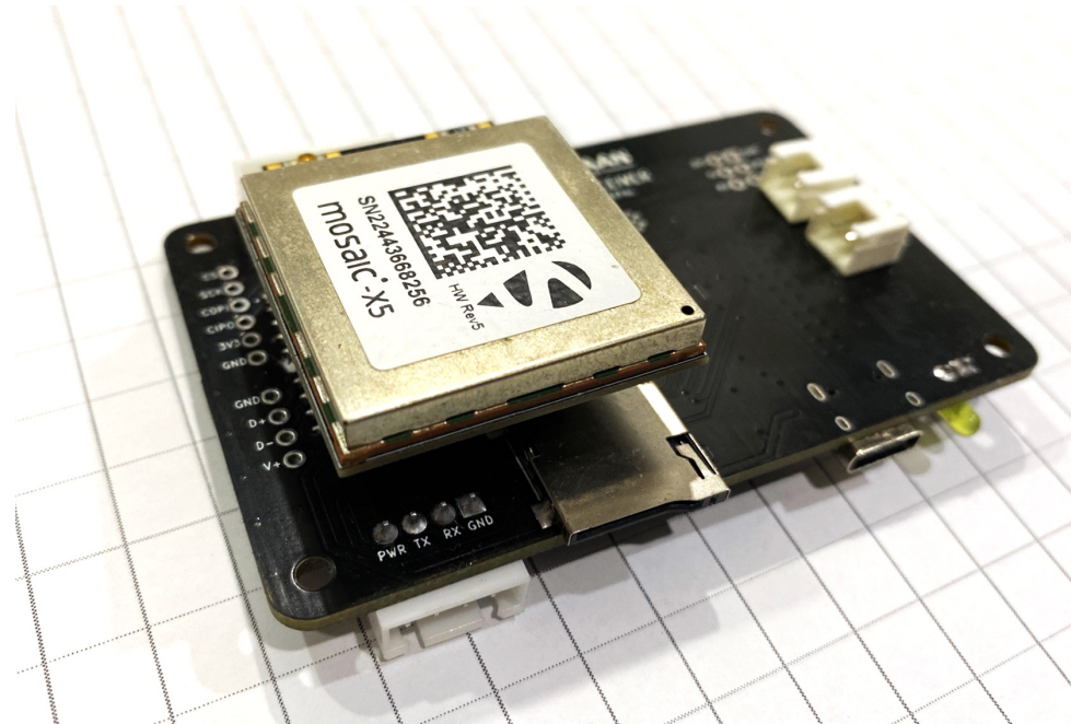
GNSS Receiver Board Upgraded with Triple-Frequency (L1+L2+L5) Receiver
