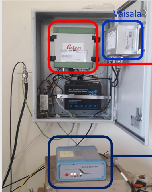
LeicaGR30 high-grade geodetic GNSS receiver
