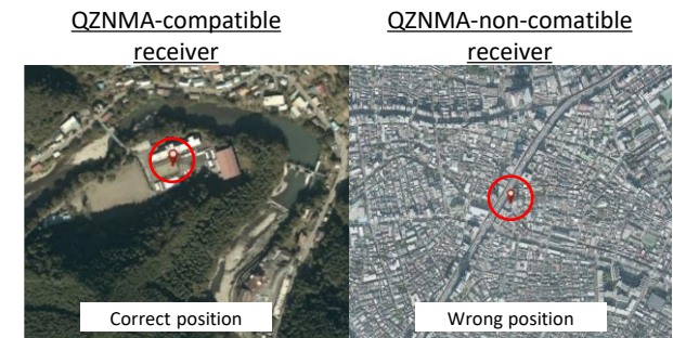
Demonstration of position being derailed by spoofing
