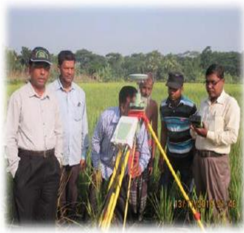
DLRS Staffs using GNSS/RTK system for Surveying in Jamalpur Sadar
