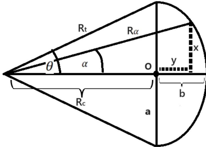
$$R_t = \frac{S}{\gamma} \ln[S\gamma(v_0 - \omega)t + 1] + \omega t + R_0$$
