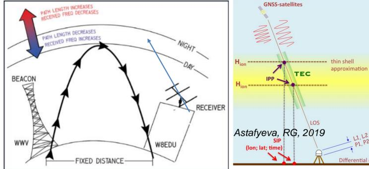
Information on wave amplitude and phase at a specific reflection point (height from ionograms) Doppler shift  $\rightarrow$  Vertical oscillation velocities of plasma/air due to the waves multi-point and multi-frequency sounding  $\rightarrow$ propagation velocities from time delays between different sounding paths
