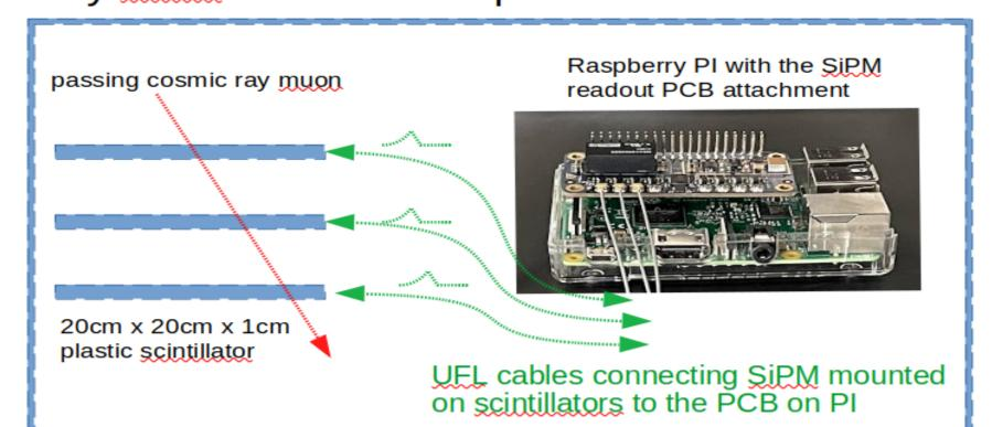
Typical detector setup at a given site. A minimum site requirement is a small desk, power and network connection. (right) Low-cost detector readout. The scintillation light generated by a passing muon particle is collected by silicon photomultipliers and the electrical signals are sent to the PCB mounted on a Raspberry Pi.
