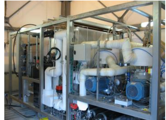
Cryogenic crystalizer breadboard for 10 crewmembers
