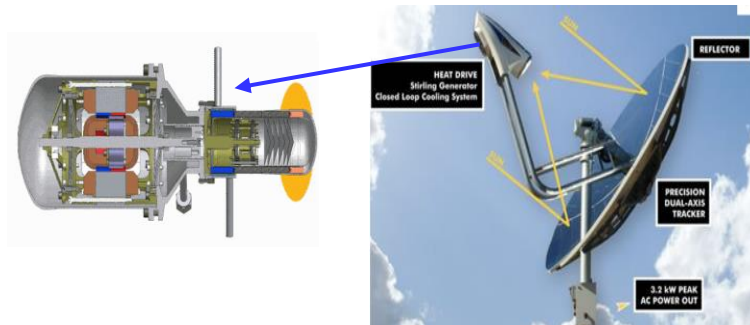
Solar Concentration Stirling INFINIA 600K – 300K
