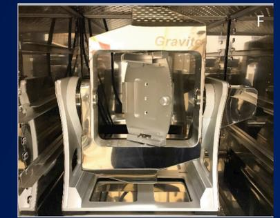
Space Bio-Laboratories, Inc. GRAVITE 3D-clinostat in an incubator
