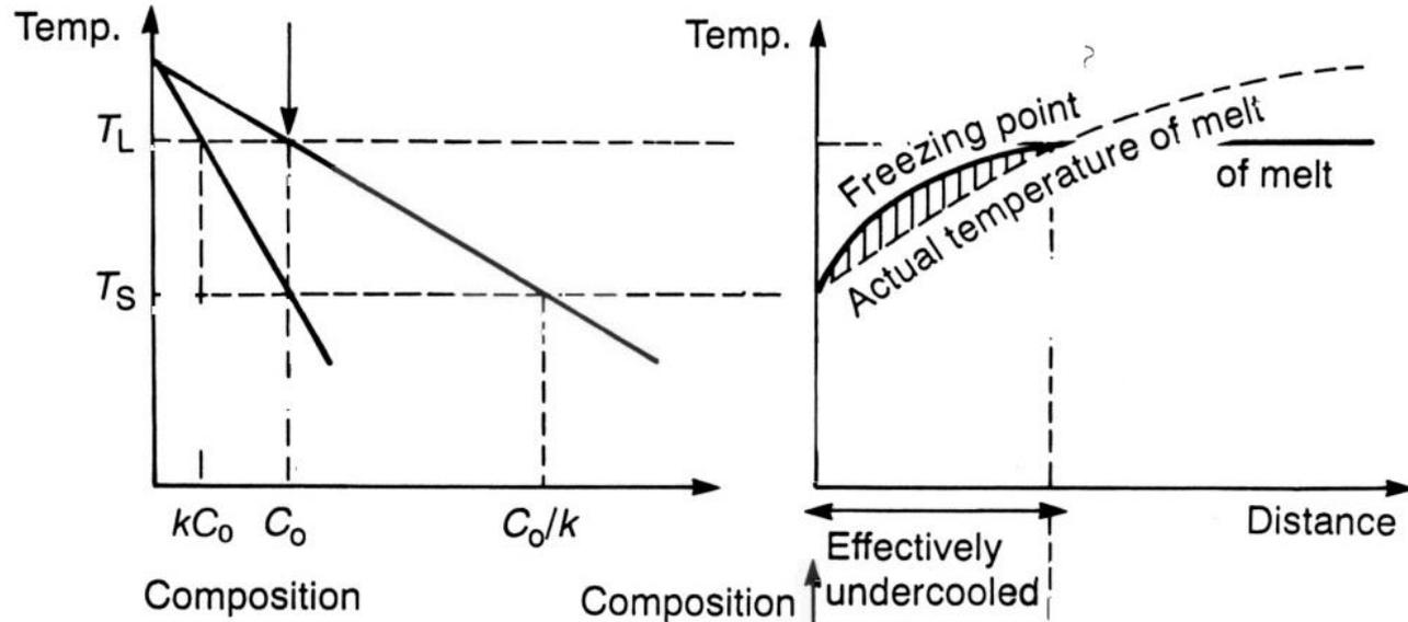
the link between the phase diagram for a binary alloy and undercooling
