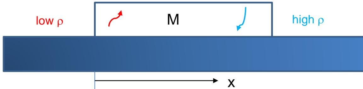
Such variations in  $T$  occurs when, for example, you're cooling a liquid metal in a mold in a casting process.
