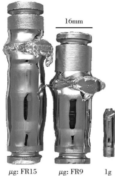
Grown crystal of GaSb both in microgravity and on earth
