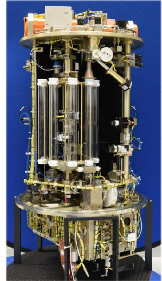
*PERWAVES experiment system with combustion tubes (Airbus D&S)*
