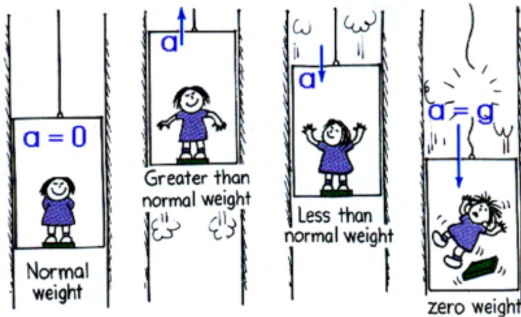
Figure: Acceleration ( $a$ ) of a body in an elevator.
