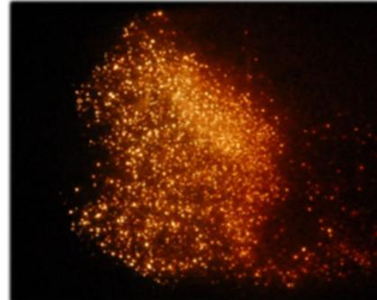
*Iron powder combustion in micro gravity*
