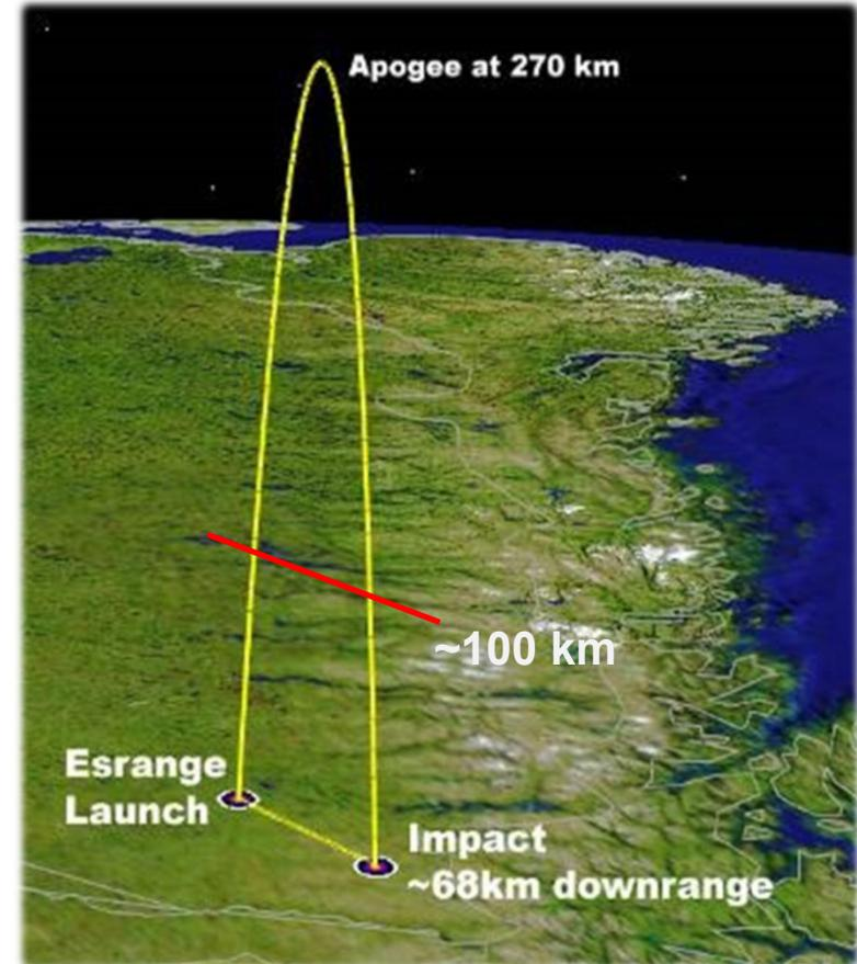
*Typical flight trajectory of a microgravity rocket .*
