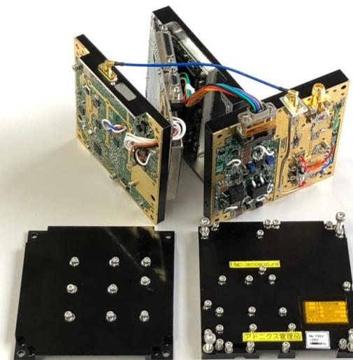
CubeSat S-band RF Transmitter and Receiver, X-band Transmitter, and inside of the X-band Transmitter (from left to right) © Addnics corp.
