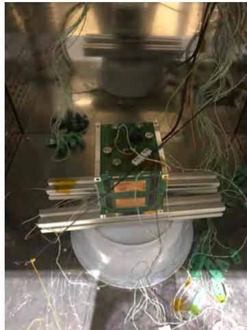
Antenna deployment in very cold temperature
