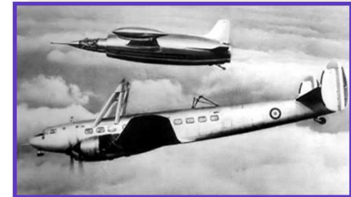
Fig. Leduc with thermopropulsive nozzle (dropped by the 'Languedoc' SE-161 carrier-aircraft) 1946-1957
