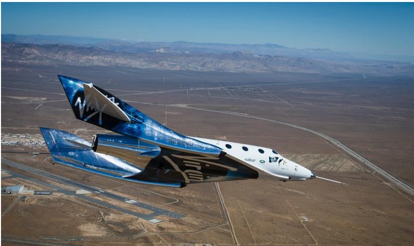
SpaceShipTwo (VSS Unity), unpowered glide test May 1, 2017. Carries 6 space flight participants, operations in 2018? Air-launched at 50,000 feet (15km) to altitude of 100km from White Knight II aircraft.
