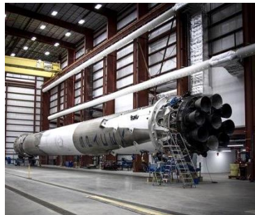
Refurbishing a first stage from Falcon 9 [photo from Jan 2016]
