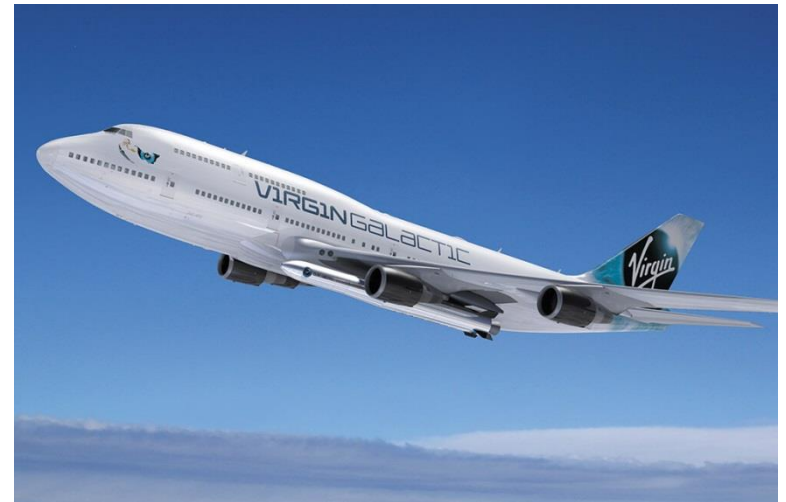
LauncherOne (concept art). Two-stage, LOX-kerosene rocket, air-launched from a 747-400 at 35,000 feet (9km).
