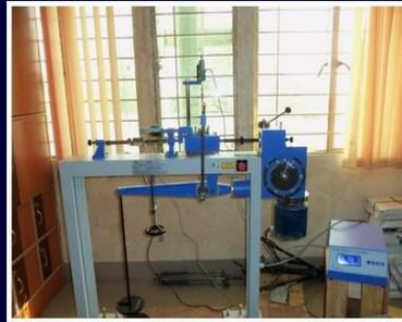
*Direct Shear Test Instrument*
