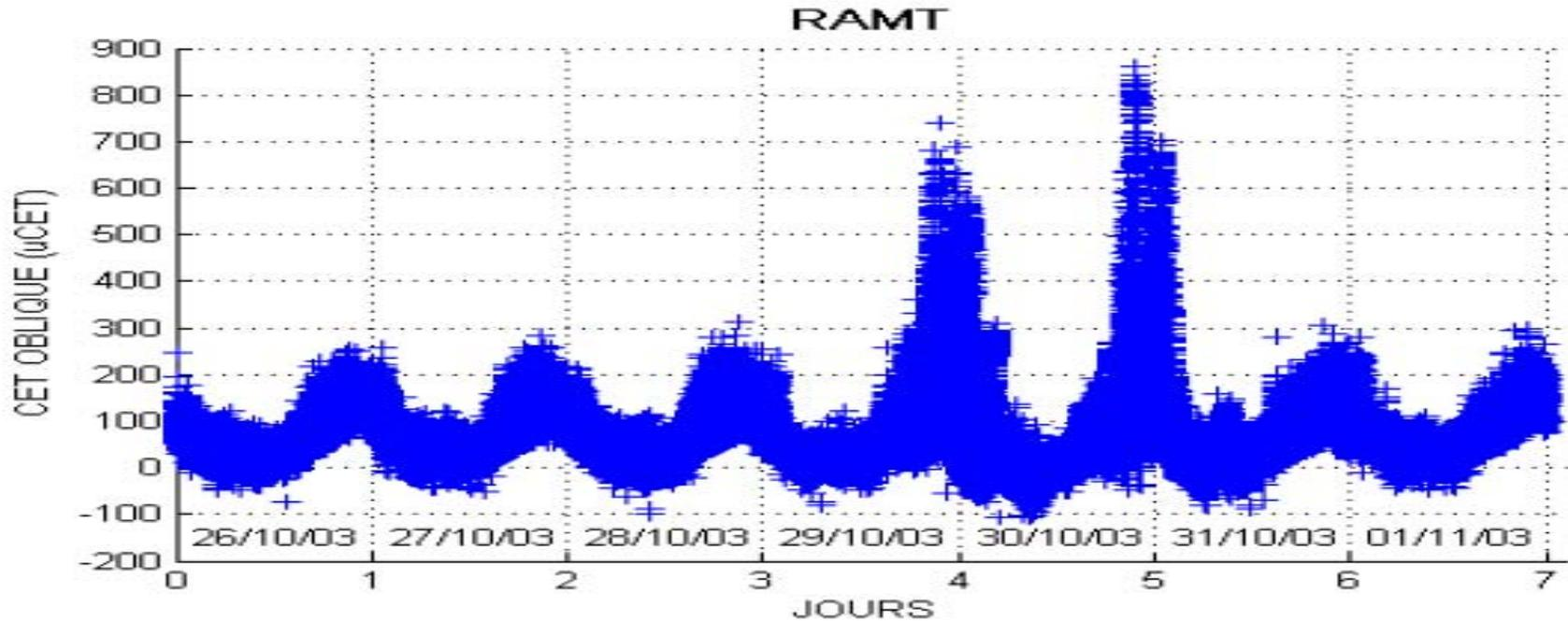
Oblique Total Electronic Content at RAMT station (USA), during a ionospheric perturbation
