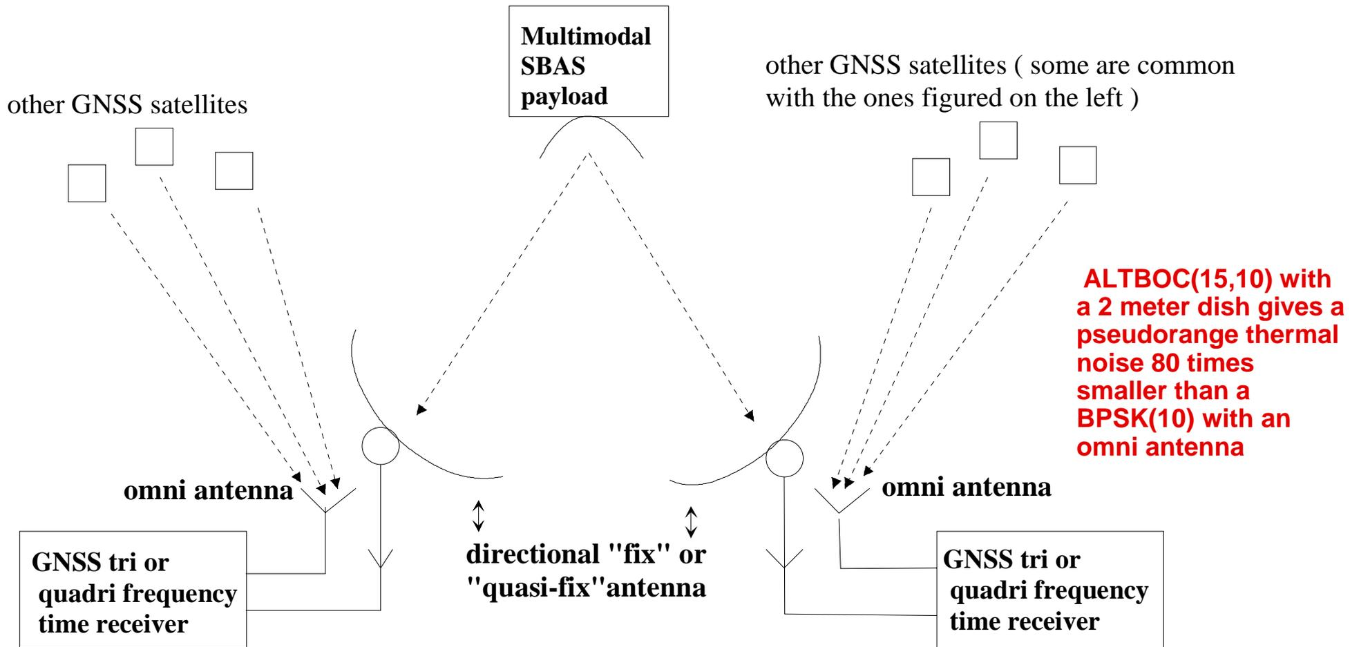
Very good accuracy offered by ALTBOC(15,x) modulations, for precise and or science applications, even when using standard omnidirectional GNSS antennas
