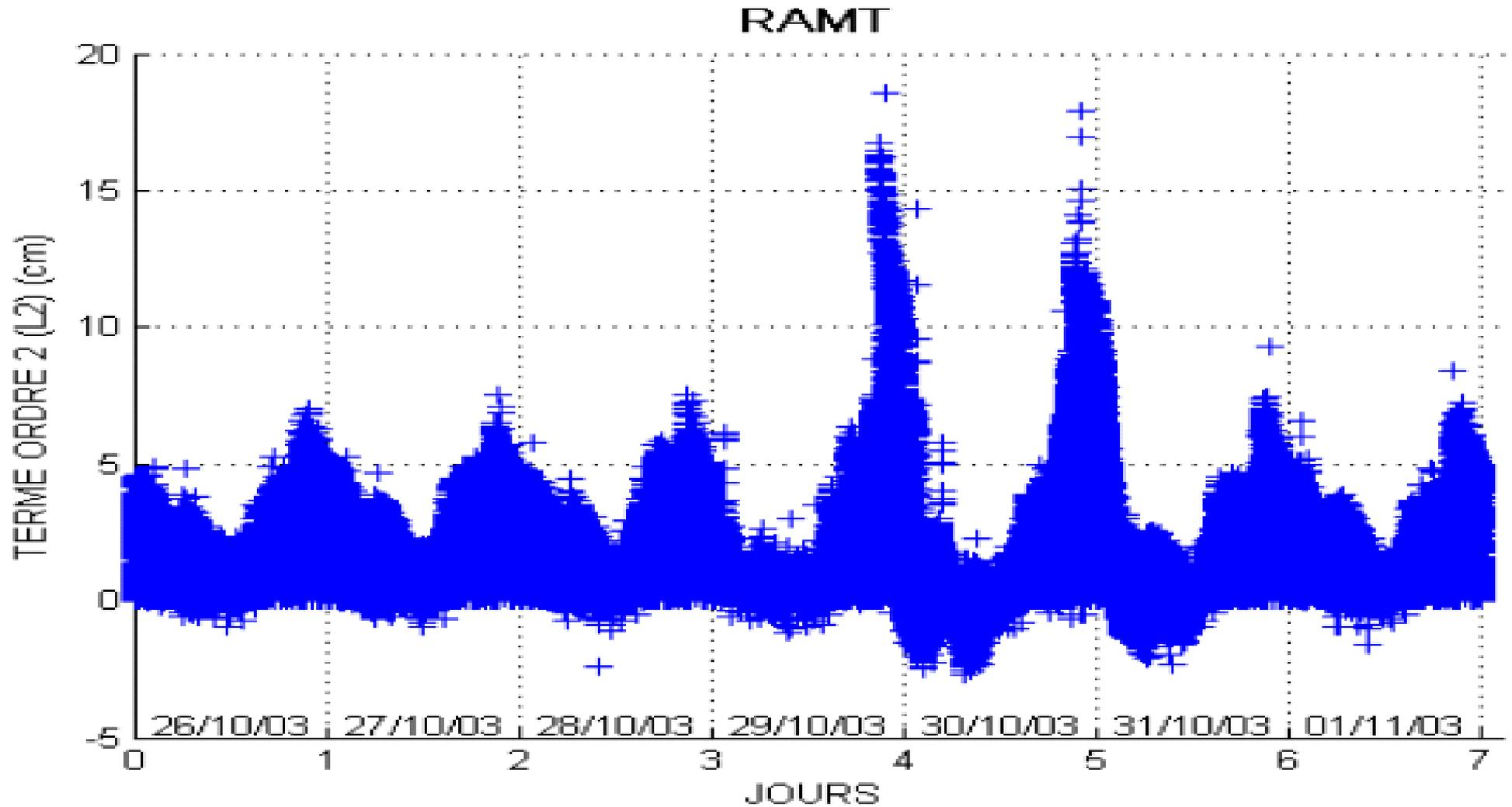
Ionospheric 2<sup>nd</sup> order pseudorange term at  $f_{NA}1$  GPS frequency calculated for the RAMT station
