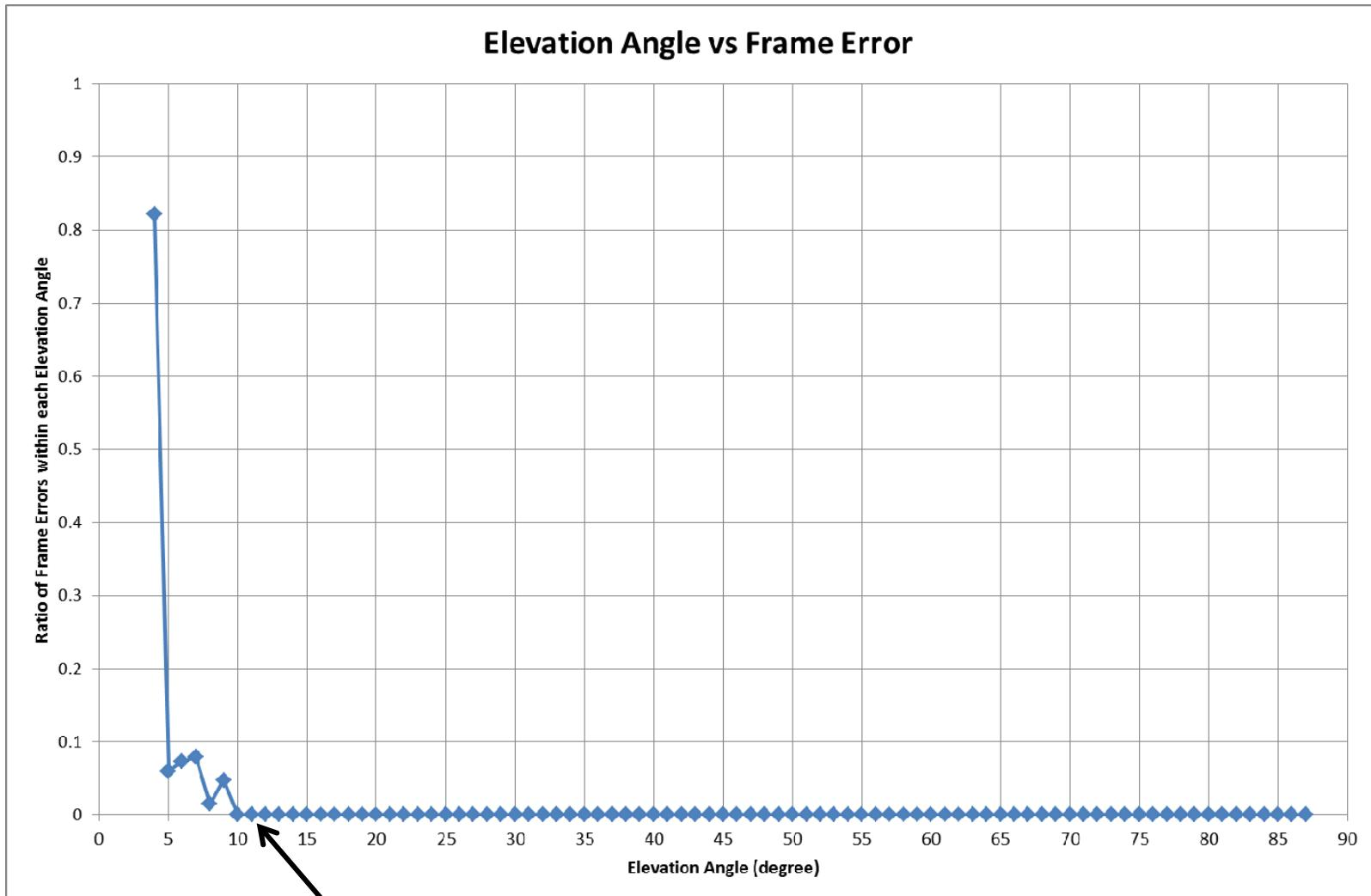
Signals at more than 10 degrees of elevation angle, No Frame Error.
