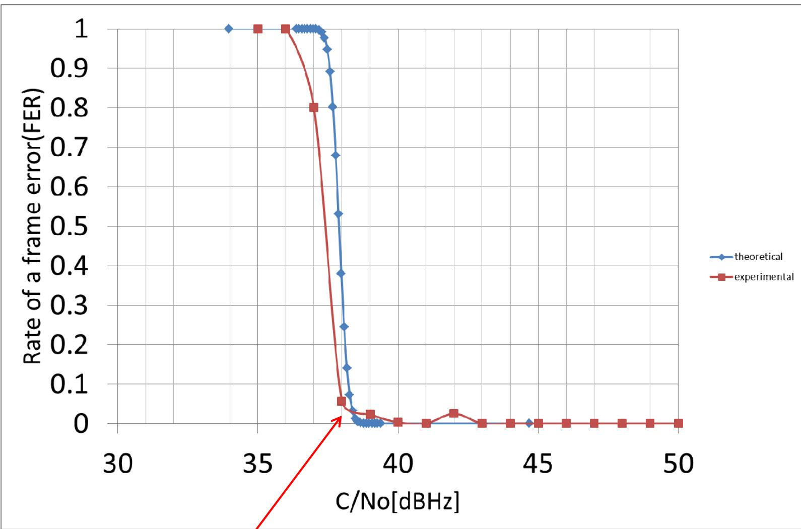
Theoretical Frame Error Rate (FER) v.s. Experimental FER is almost same.
