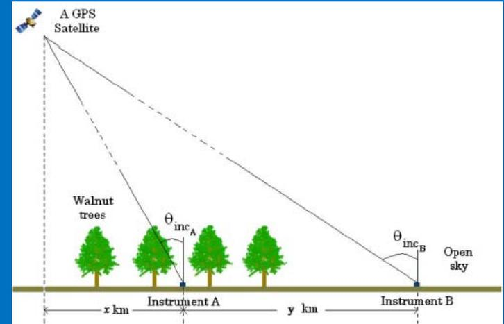
Experimental setup. Instrument A, deployed under trees, and instrument B, deployed under open sky, simultaneously measure GPS signals.
