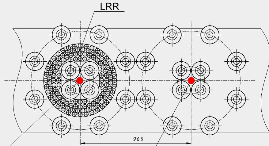
Phase center of antenna transmitting L1OC, L1SC, L2SC, L2OC, L3OC navigation signals
