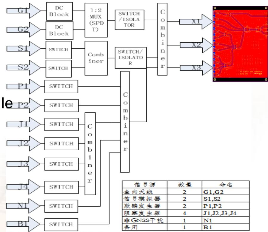
**Internal logic diagram of RF switching and overlay module**
