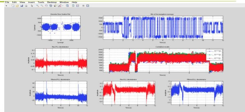
Influences of the Spoofing interference on the tracking loop
