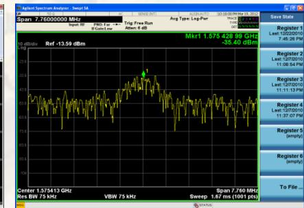
The spectrum of 8 GNSS spoofing signals
