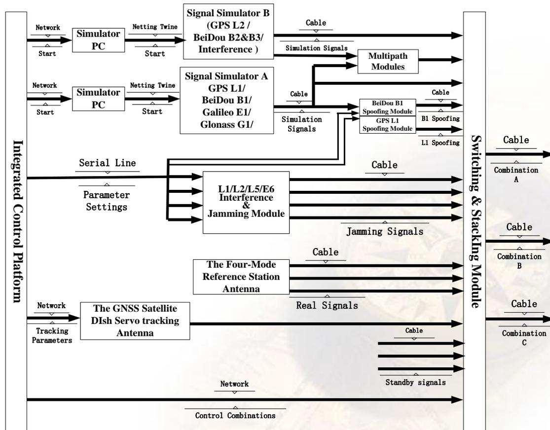
Signal-In-Space Environment Simulation Subsystem
