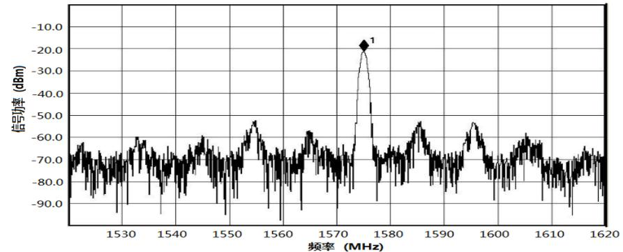
**Obstruction spectrogram of single-frequency interference produced by the jamming device**
