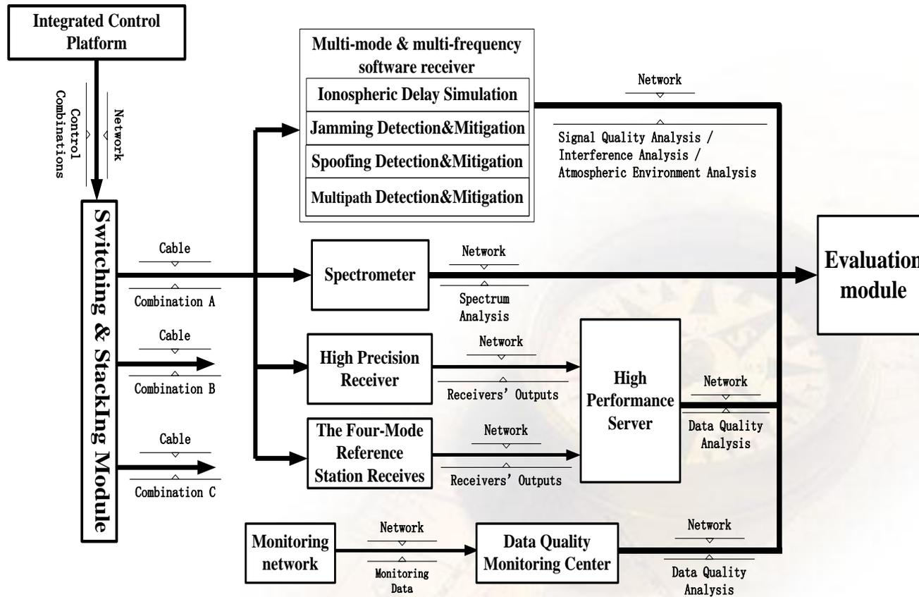
Signal Processing And Quality Monitoring Subsystem
