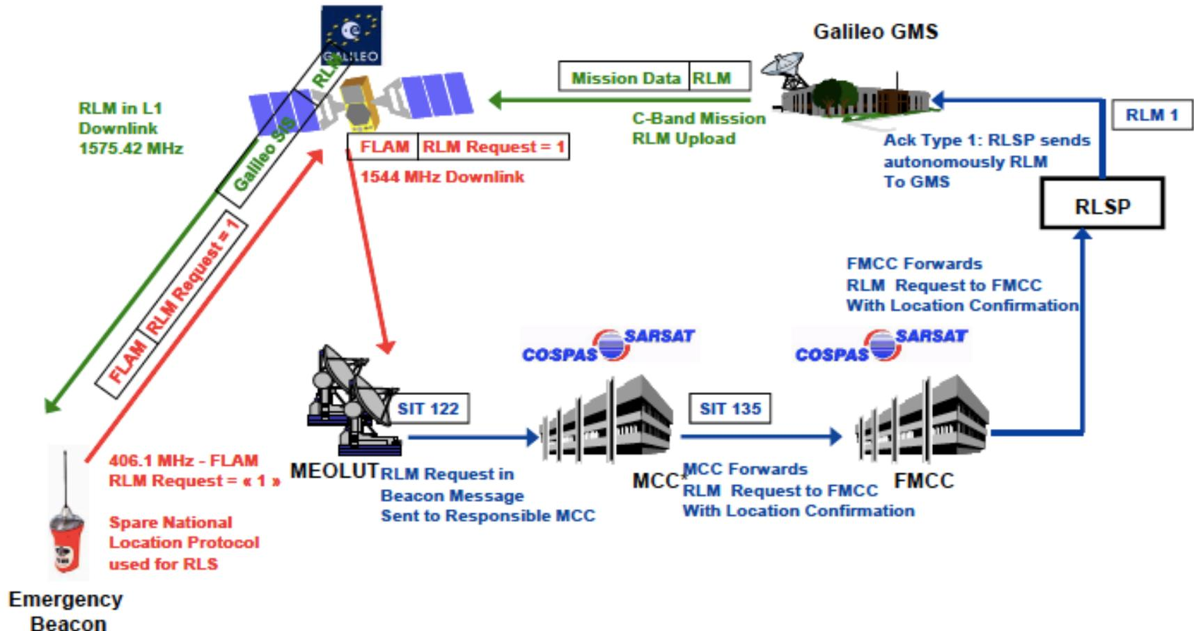
Message sent by the distress beacon (specific RLS protocol on the 406 MHz uplink signal) to the RLS Provider (RLSP) to indicate it has a Return Link capability
