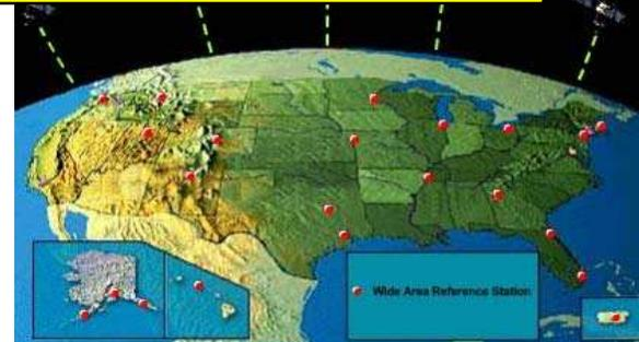
Correction messages for atmospheric, orbit & sat clock errors (via GEO "GNSS-like" satcom link)
