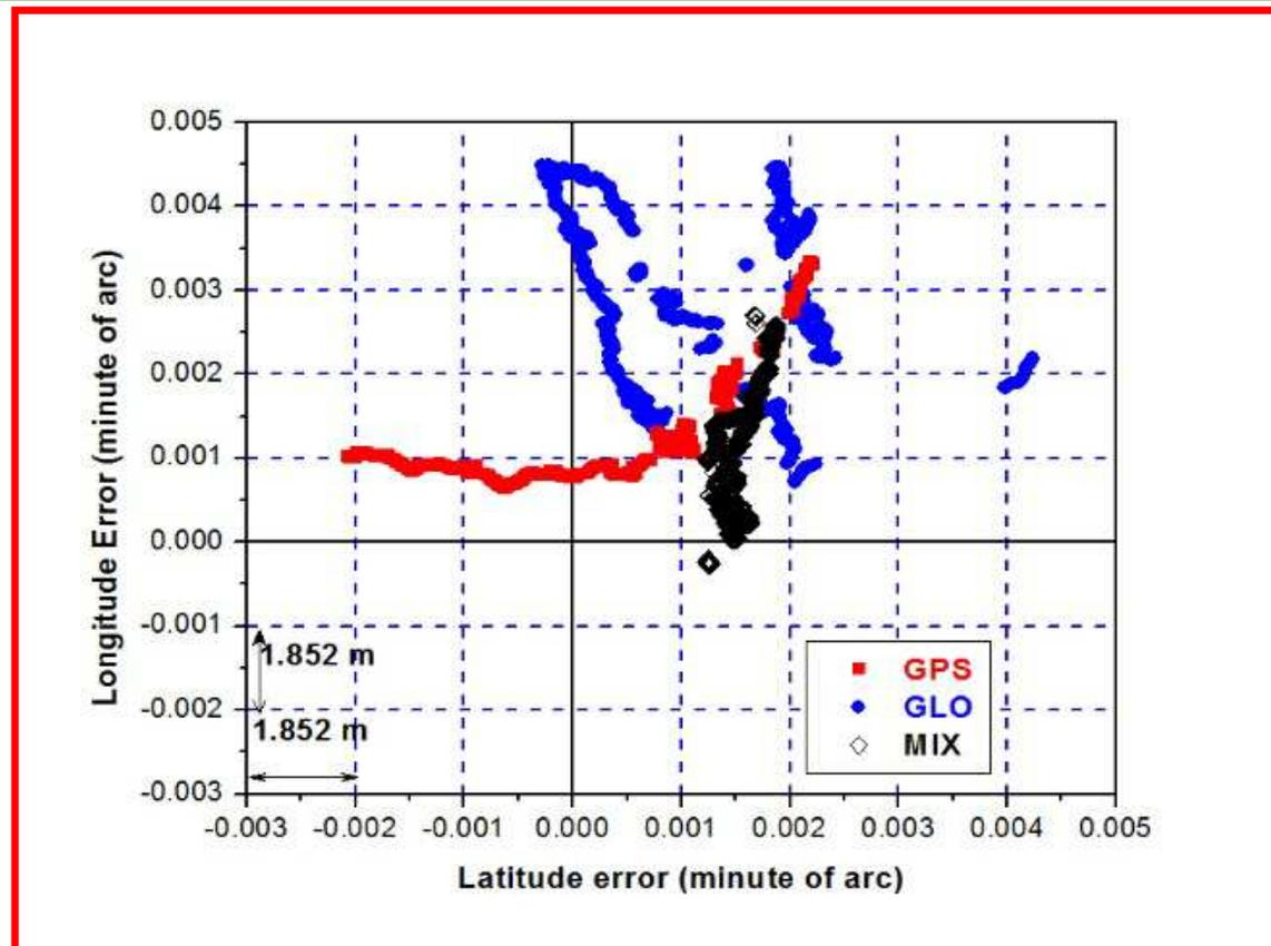
1 hour data @ 1 Hz each for GPS, GLONASS, GPS+GLONASS
