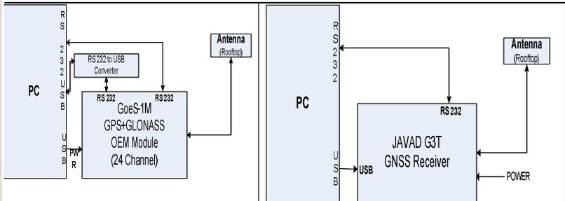
Experimental setup for GoeS-1M receiver
