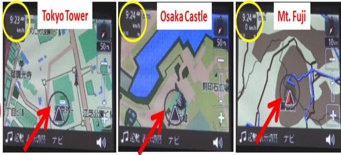
Spoofers transmit signals similar to signals from satellites. The receiver can't distinguish between the SPOOFER signal and Satellite Signal.
