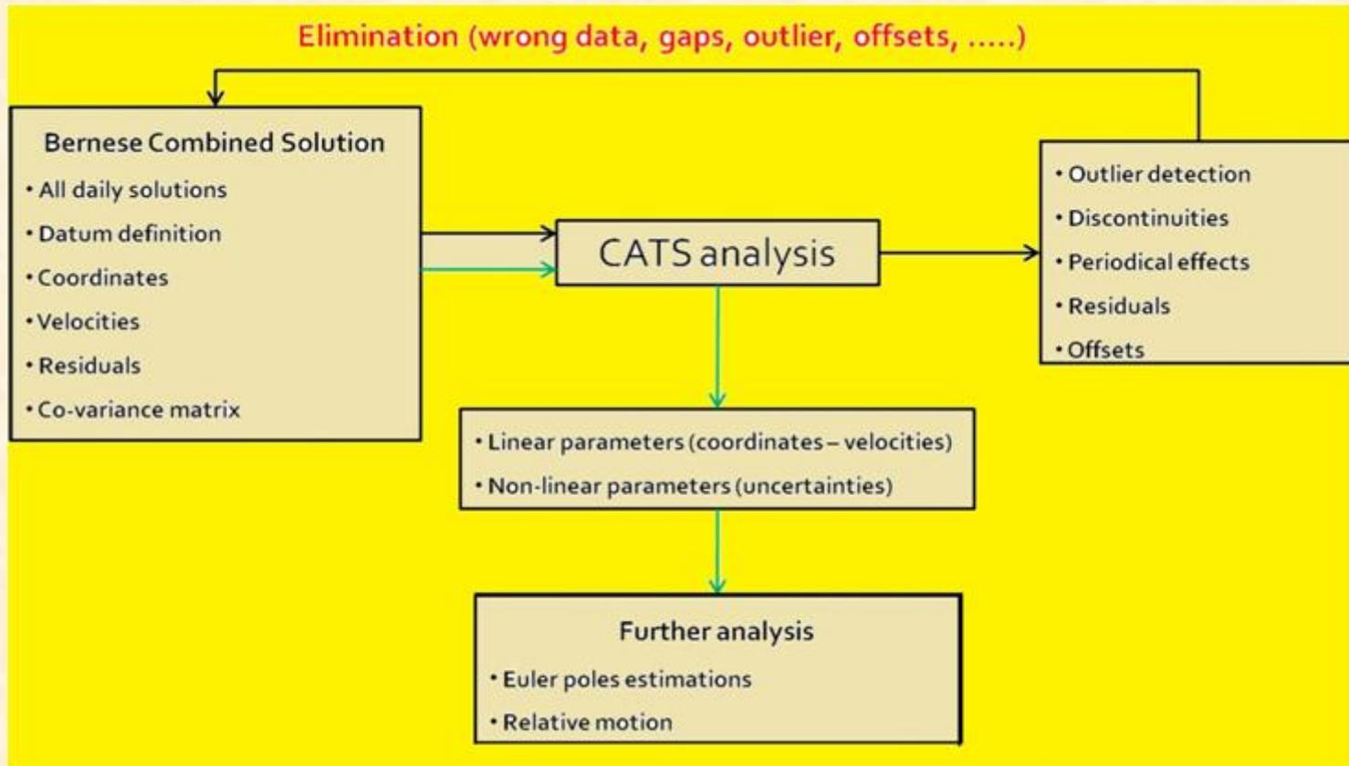
**Flow diagram of the CATS processing scheme**
