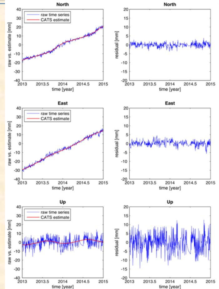
Bernese raw time series (blue line) and the estimated CATS time series (red line) in the left side and residual in the right side in each component using white noise plus power law noise model for stations PHLW (a) and KLHV (b).
