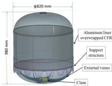
Fig.-9 Concept of CFRP propellant tank
