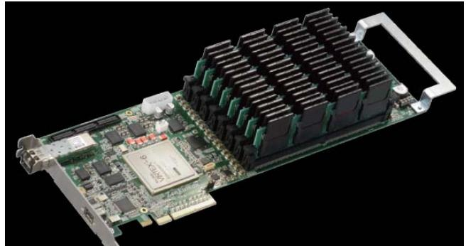
**Fig.-3** The FPGA board manufactured by Technoscope which can analyze 32 4K4K-frames with 40 seconds.
