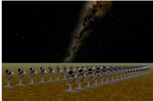
**Fig.-2** The array of the optical sensor at one site. In order to detect many LEO objects two times, two narrow rectangle regions are observed by changing observational direction of each optical sensor.
