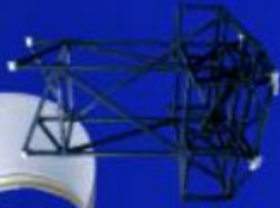
Launch vehicle aft sections and spacecraft trusses made of carbon fiber composite
