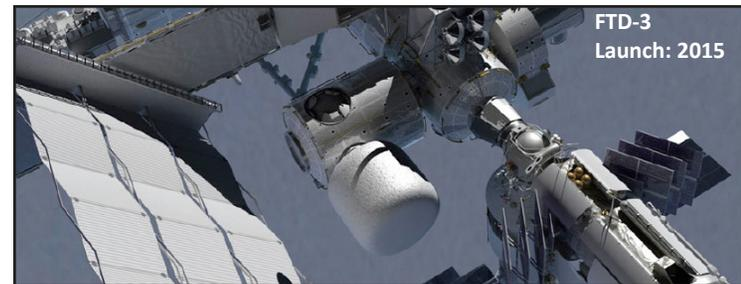
Inflatable ISS mission module, with Closed-loop Environmental Control and Life Support (ECLS)
