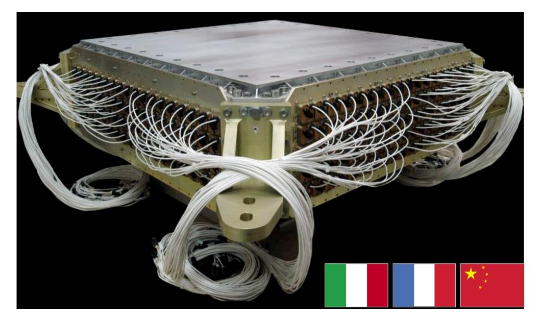
50,000 fibers,  $\phi = 1$ mm, distributed uniformly inside 1,200 lb of lead which provides a precision, 3-dimensional,  $17X_0$  measurement of the directions and energies of light rays and electrons up to 1 TeV
