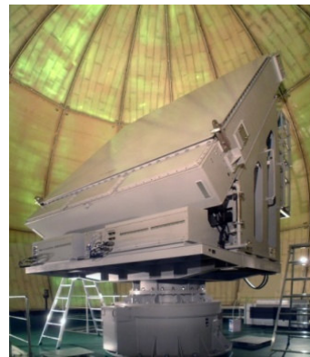
Kamisaibara (KSGC) Radar / Japan Space Forum Detestability: 1m \phi at 577km
