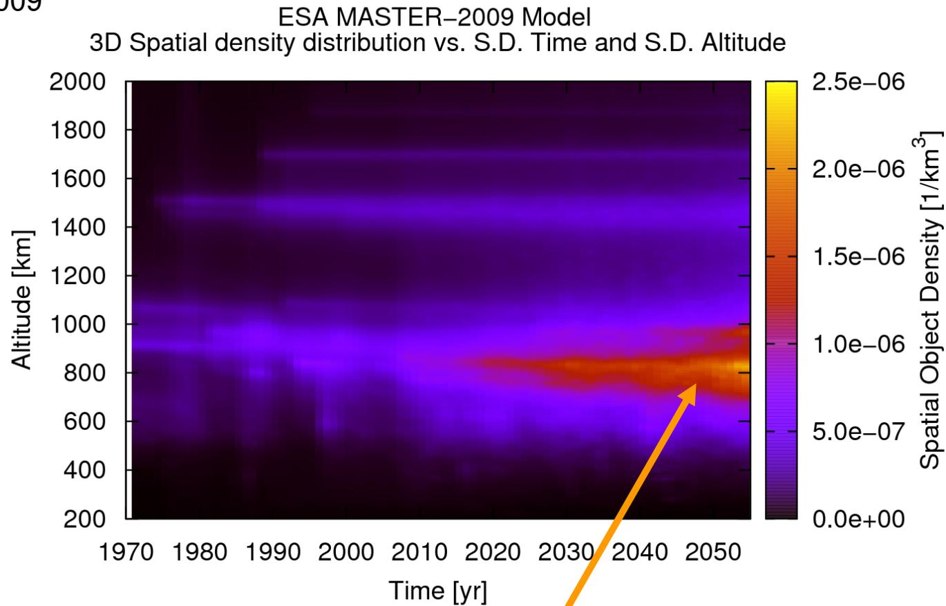
**Increasing threat for the orbits used by Earth observation satellites**
