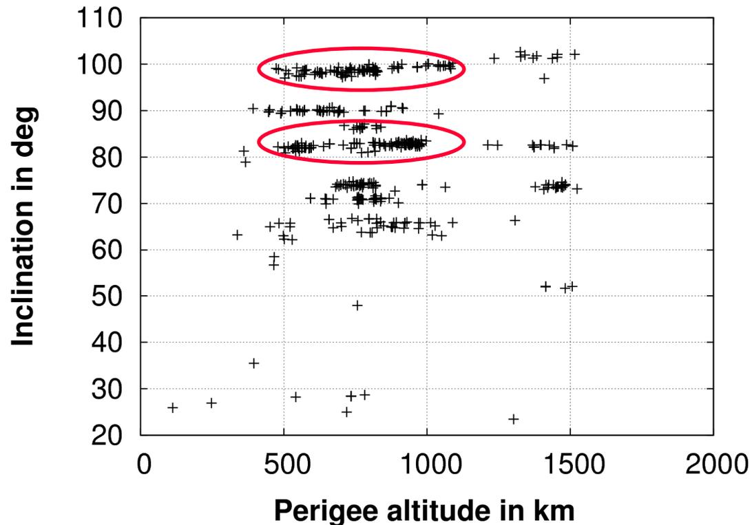
Collisions will mainly occur between sun-synchronous satellites ( $i \approx 98^\circ$ ) and objects at  $i \approx 82^\circ$ . Basically head-on collisions with twice the orbital velocity!
