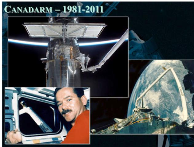
The original Canadarm was capable of deploying or retrieving payloads weighing up to 332.5 kg (733 lb) in space. In the mid-1990s the arm control system was redesigned to increase the payload capability up to 3,293 kg (7,260 lb) in order to support space station assembly operations.
