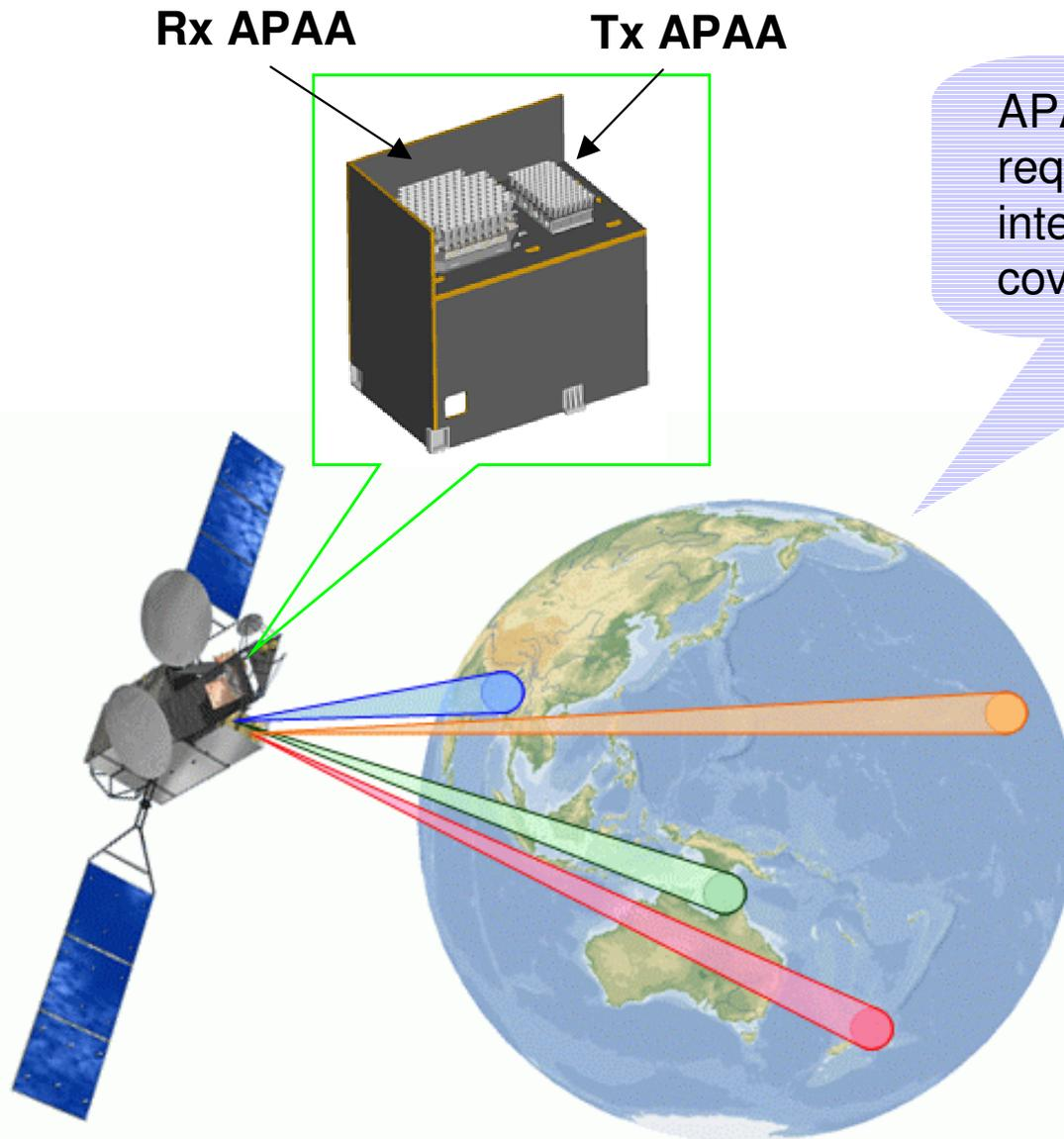
APAA can hop its beams to required points in 2msec interval to provide a wide coverage area.
