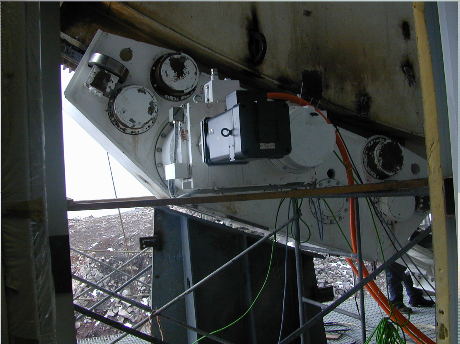
The elevation drives tested and working
