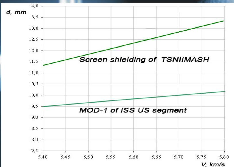
**Experimental data comparison on ballistic limit curves of ISS US segment shielding MOD-1 and TSNIIMASH shielding**
