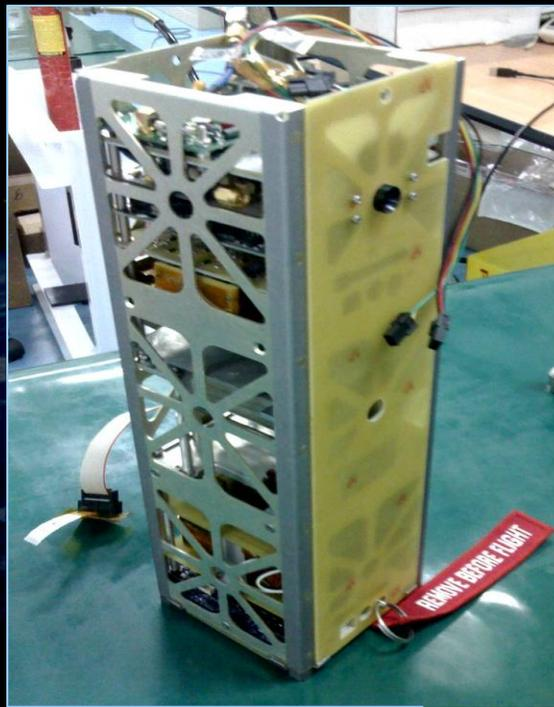
CubeSAT FM during camera test
