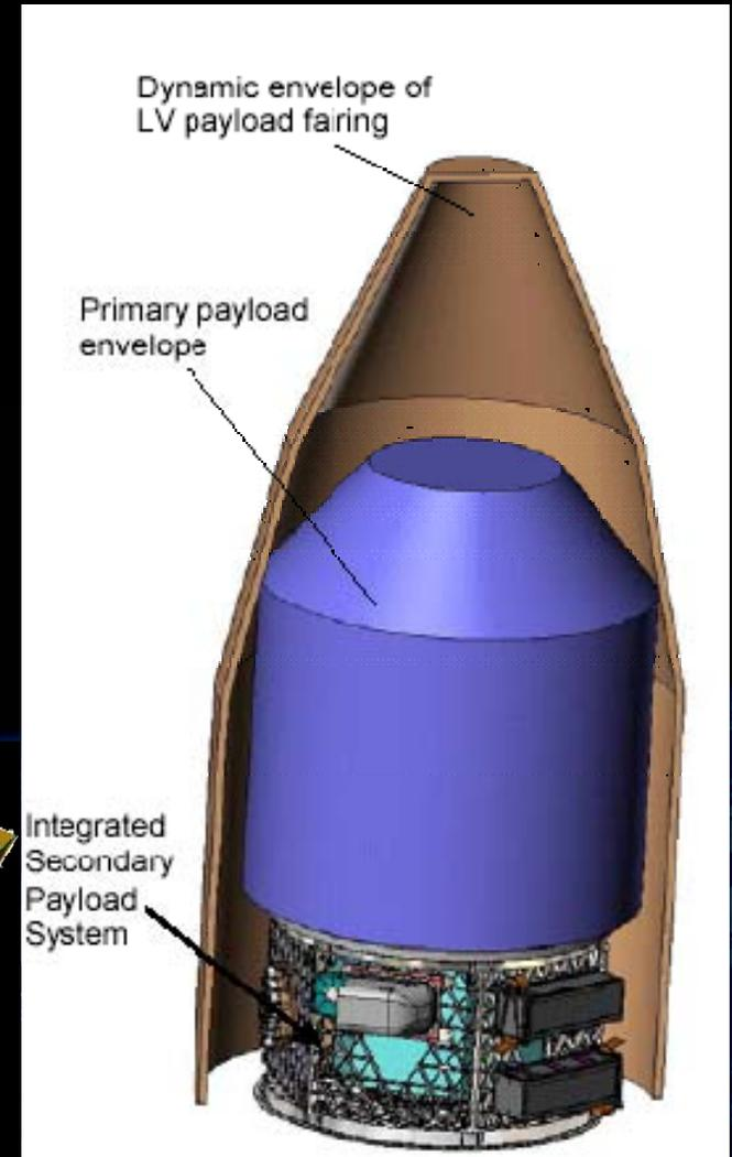
Secondary Payload Adapter and Separation System
