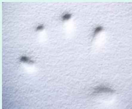
Initially referred to as “slow spring back foam,” temper foam matches any pressure against it and slowly returns to its original form once the pressure is removed.
