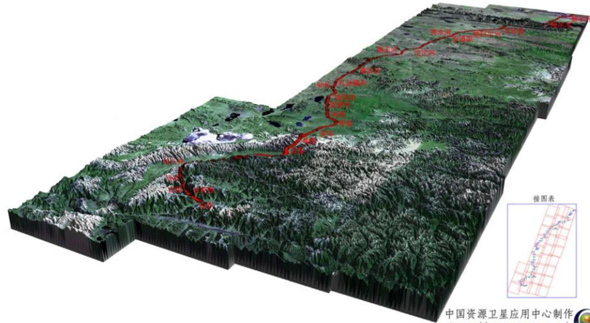
Three-dimensional image map for Qinghai-Tibet Railway, resulting from data of CBERS-2 CCD camera and 1:250000 DEM data
