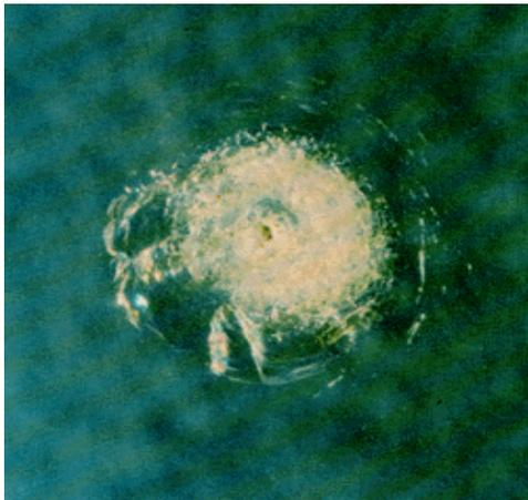
**4-mm-diameter crater on windshield of Space Shuttle Orbiter made by 0.2 mm fleck of white paint; relative velocity at impact: 3-6 km/sec (NASA photo)**
