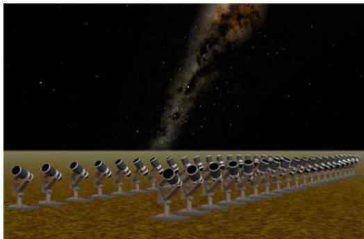
**Fig.-2 The array of the optical sensor at one site. In order to detect many LEO objects twice, two narrow rectangle regions are observed by changing observational direction of each optical sensor.**
