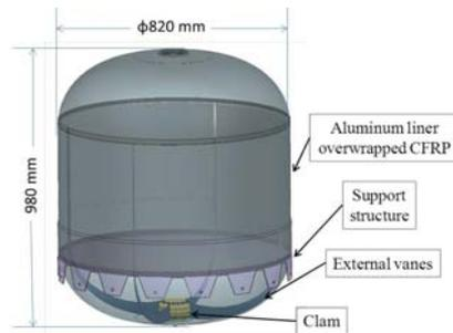
**Fig.-9 Concept of CFRP propellant tank**
