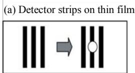
(b) Strips severed by debris particles
