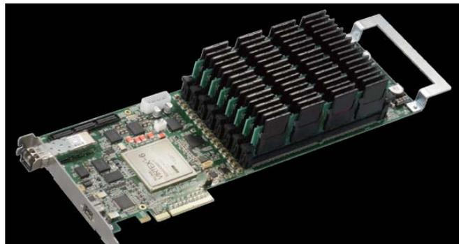
**Fig.-3 The FPGA board manufactured by Technoscope which can analyse 32 4K4K-frames within 40 seconds.**
