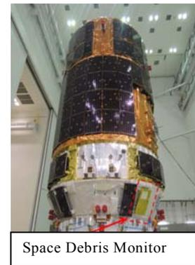
Fig.-6 Flight experiment on HTV
