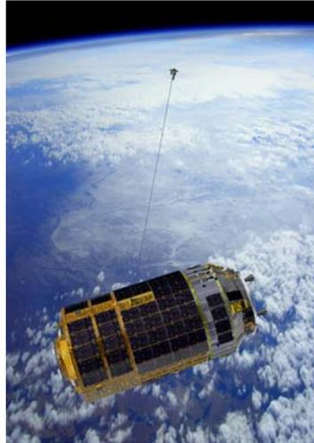
**Fig.-11 A demonstration flight of EDT using HTV-6**
