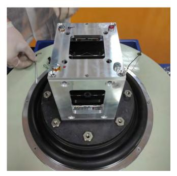
TUMnanoSAT of Moldova going under the vibration test. Credit: Technical University of Moldova
