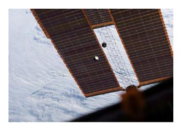
1U CubeSats Irazu (Costa Rica) and 1KUNS-PF (Kenya) deployed from the JEM Small Satellite Orbital Deployer. The 1KUNS-PF (Kenya) CubeSat was deployed under the Access to Space for All Initiative. Credit: JAXA/NASA
